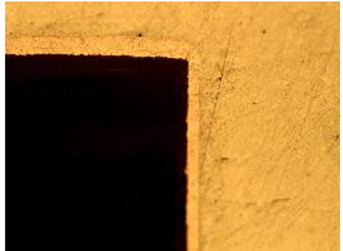
Figure 15. 6x Solder Shock at 200x magnification
