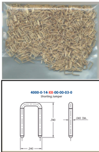
Figure 2. Investigation Test Components (Top: As Received Parts, Bottom: Jumper Dimensions)
