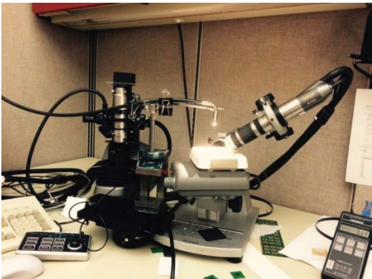
Figure 7: Keyence video microscope configured with hot plate.
