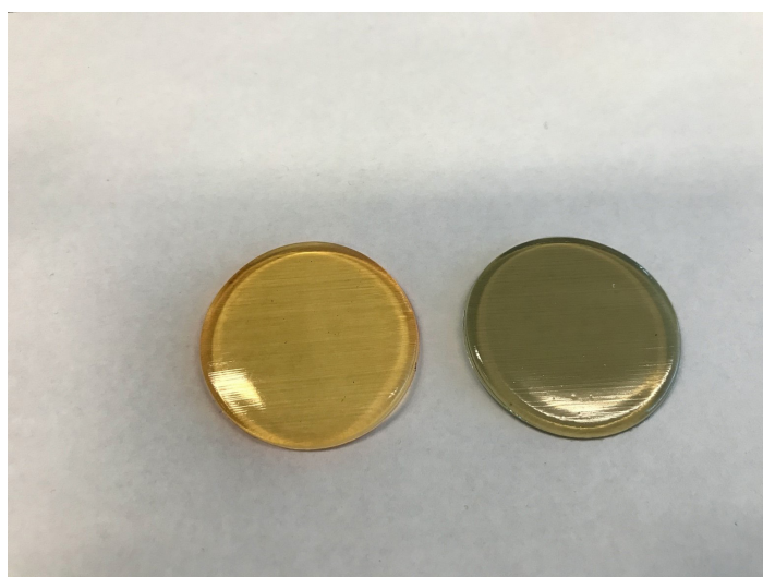
Figure 3: Examples of printed materials (D = 36 mm). Left: C3-DI-7. Right: C3-DI-7-CNT (mix of C3-DI-7 and C3-DI-CNT).
