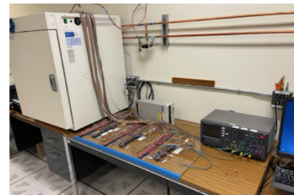
Figure 2: (a) 10 daughter cards plugged in to a motherboard; (b) over all view of test setup.
