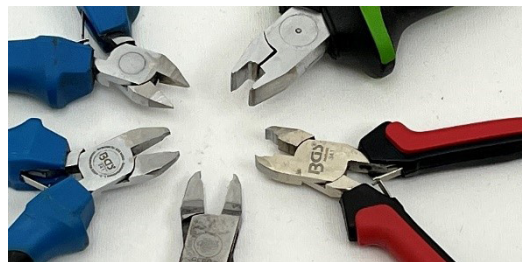
Figure 2: Special pliers for tearing components. Each can be used only for a specific type of component.
