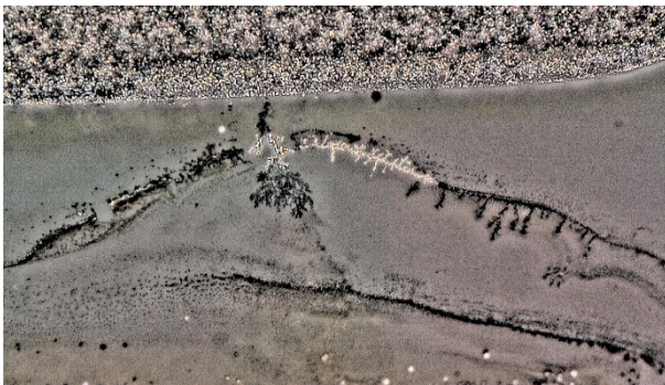
Figure 18: Details of the Dendritic structure of Silver, grown in flux residues during the moisture test 90%rH, 40°C, 169 hrs.
