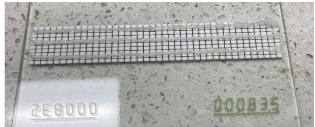
Figure 8: Deposit of solder paste flux before reflow
