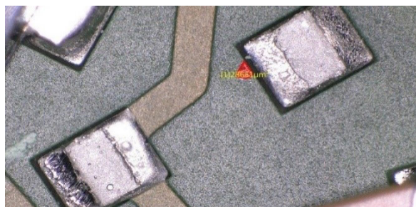
Figure 3: A trained person can tear the component of the board without board damage
