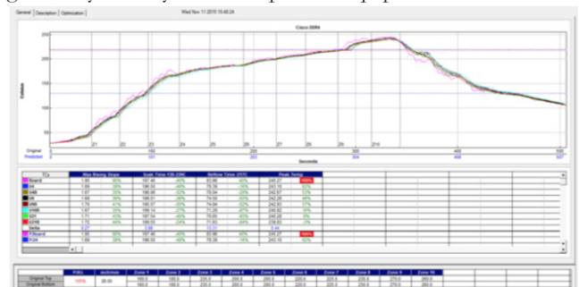
Figure 5a: DDR4 TV Reflow Profile
